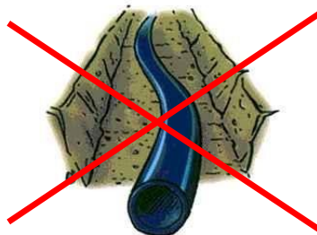
Wrong: vertical or horizontal ripple The waviness of the trench bottom was not compensated for here and is therefore transferred to the pipe structure. A reduction in the blowing length is to be expected!
