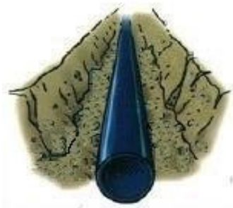
Correct: straight pipe laying If possible, the pipes should be laid under tension.
